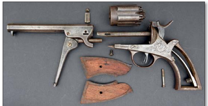
Engraved Walsh 12-Shot "Navy" Revolver s/n 117 Exploded View
