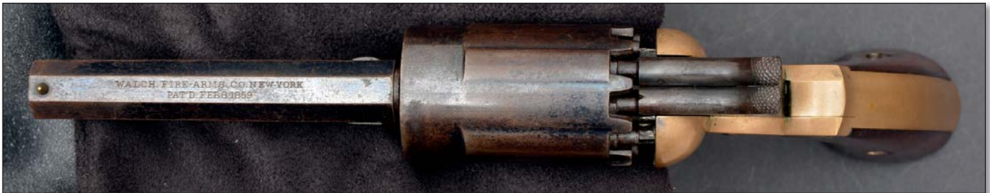
Walch 10-Shot Pocket Revolver s/n 1338 - Note double hammers with sighting groove on left hammer
